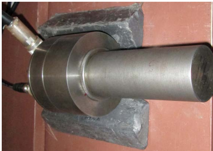
Figure 5 Re-purposed Beryllium Rod Detector Housing
